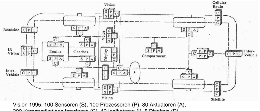
200 Kommunikations Interfaces (C), 40 Indikatoren (I), 5 Displays (D), 4 Vision Systeme (V)
