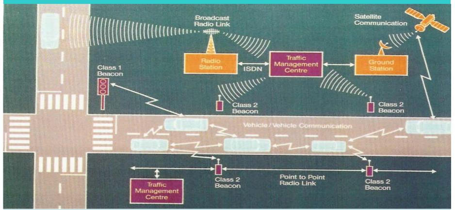
Pro-Net: Development of a communication network between vehicle- computers, enabling the vehicle to be driven safely by means of "electronic sight", increasing the perception area of the driver.
