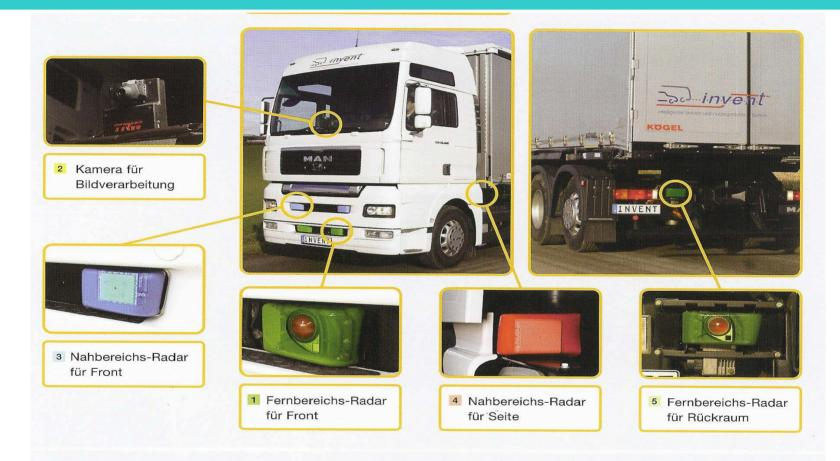
Test- Vehicle of MAN: 77 GHz front and rear end radar, 24 GHz short distance radar,Camera Systems. Sensor Fusion + Pattern recognition+ Environmental Models+ Validation + Interpretation of Situations.
