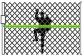
The function of a barrier system is to restrict, deny, delay, or channel the flow of pedestrian or vehicular traffic to a site. Barriers are not impenetrable but increase the probability of detecting persons or vehicles attempting to gain unauthorized access onto a site or dissuading them from attempting access. They offer a time delay to allow your security force or employees to detect and possibly assess illegal intrusion or trespassing.
