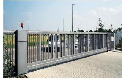
Retractable barrier systems may be portable and can be placed during periods of increased threat levels and later removed. The selection and application of gate barriers depends on the size and speed of the anticipated terrorist vehicle. Speed bumps or a serpentine entrance can reduce vehicle speed.
