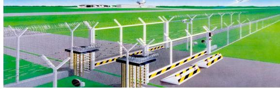
Entrapment areas can also use mechanical turnstiles or gates to isolate entry to one individual at a time. In addition to electronic access by users, a security officer or member of the facility staff may operate the entrapment area gate electronically or manually.
