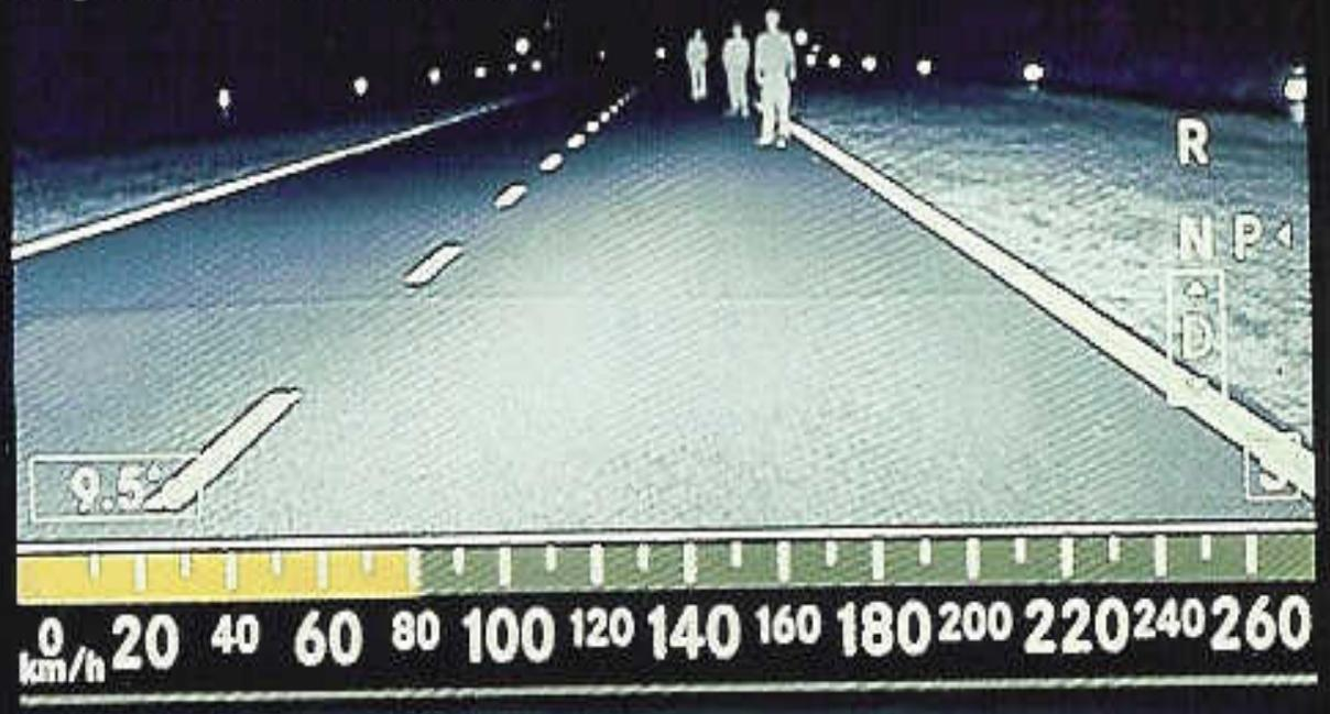
2005 Series Production of Night Vision Systems enhancing the Vision of the driver at night of up to 150 meter.
